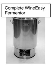
**IMPORTANT:** Prior to assembling the fermentor it is important to ensure that the tank has not been bent from shipping. Use a tape measure to check for circularity – the difference in inside diameter all around the tank should be less than 1/8". If it is slightly out of round, simple lay the fermentor on its side and push gently to reshape it. Otherwise contact your retailer.
