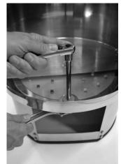
wrench on the outside. Do NOT use Teflon tape on these threads! Note that the wrenches are not supplied.
