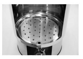
Install the screw-eye in the false bottom as shown. This is used as a handle to remove the false bottom after use, and then place it on the bottom of the fermentor. Use the large fender washer and wing nut to secure it to the bottom of the fermentor. Finger tight is plenty – do not over tighten.
